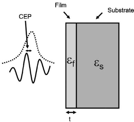
Fig. 1. Schematic of the light-matter geometry. An ultrashort several-cycle optical pulse comes in from the left and excites a nonlinear thin film of thickness  $t$ , where the film and substrate have optical dielectric constants,  $\epsilon_f$  and  $\epsilon_s$ , respectively.
