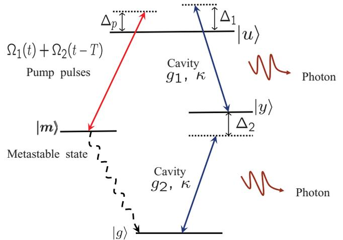
FIG. 1. (Color online) Schematic diagram for time-bin entangled photon generation. The transitions from the biexciton state  $|u\rangle$  to the exciton states  $|y\rangle$  and  $|y\rangle$  to ground state  $|g\rangle$  are coupled by a  $y$ -polarized cavity mode. The QD is pumped from the metastable (or long lived) state  $|m\rangle$  to the biexciton state through the superposition of two input pulses.
