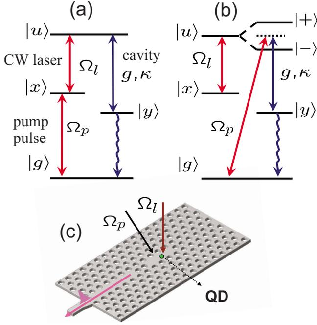
FIG. 1. (Color online) (a) Schematic of the single photon source exploiting the Raman flip process in a QD, using a CW-control laser and a pump pulse laser, and (b) the equivalent scheme in a dressed state picture. (c) Schematic of an example on-chip single photon source using a planar photonic crystal system (see Refs 26 and 27); other examples, e.g., could include the semiconductor micropillar systems (see Refs. 22 and 23).
