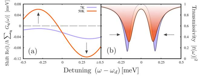
FIG. 5. (Color online) (a) Phonon induced renormalization of the resonance frequency for 7 and 50 K. The gray line marks zero shift. Below (above) the QD resonance, a positive (negative) shift is found. (b) Corresponding transmission spectra featuring a narrower VRS with higher temperature.
