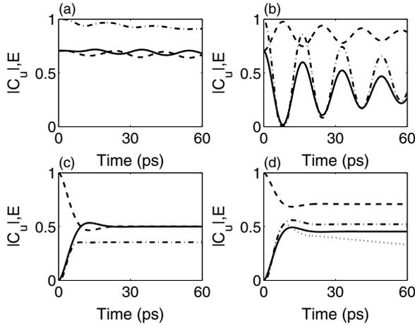
FIG. 3. (a) Upper decay of the entangled quantum dots  $a$  (solid curve) and  $b$  (dashed curve), and the entanglement  $E$  (chain curve); the QDs are detuned by 0.1 meV. (b) As in (a) but with  $d_a = 1.6d_b$  and no detuning between the dots. (c) Equal dipole moment QDs in a reduced  $Q$  cavity (factor of 10 smaller than the above). (d) As in (c) but with  $d_a = 1.3d_b$ ; the dotted curve shows  $E$  with 0.1 meV detuning between the QDs.
