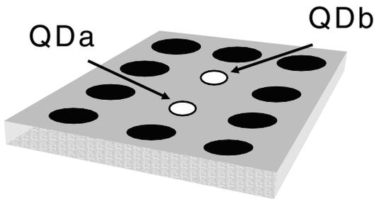
FIG. 1. Simple schematic of a semiconductor PPC nanocavity. The holes represent etched air holes, and a deliberate missing hole forms a defect nanocavity; two quantum dots (QDs) are embedded near a field antinode that contains one electron-hole pair in the spectral region of interest. In reality, of course, the PPC contains many more holes.
