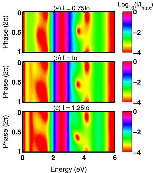
FIG. 3 (color online). (a–c) Contour “phase maps” of the emitted field 1 cm from the semiconductor, for several different incident intensities.
