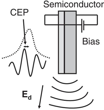
FIG. 1. Schematic of the light-matter excitation scheme. An ultrashort several-cycle optical pulse, with a specific phase (CEP), excites a large density of carriers in the semiconductor thin film. When electrically biased, even weakly, this results in the emission dipole-induced electric field propagating in the far field.
