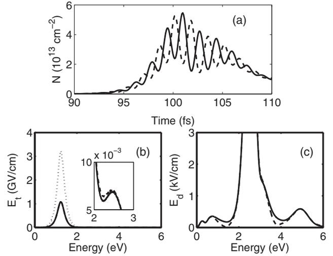
FIG. 2. (a) Electron-hole sheet density versus time for two different values of CEP (solid and dashed curve). (b) Incident field (dotted curve) and transmitted field using the same phases as above (solid and dashed curve); also shown as an inset is an amplified spectral region of the low intensity changes that have taken place. (c) Emitted field from the time dependent dipole, 1 cm away from the sample.
